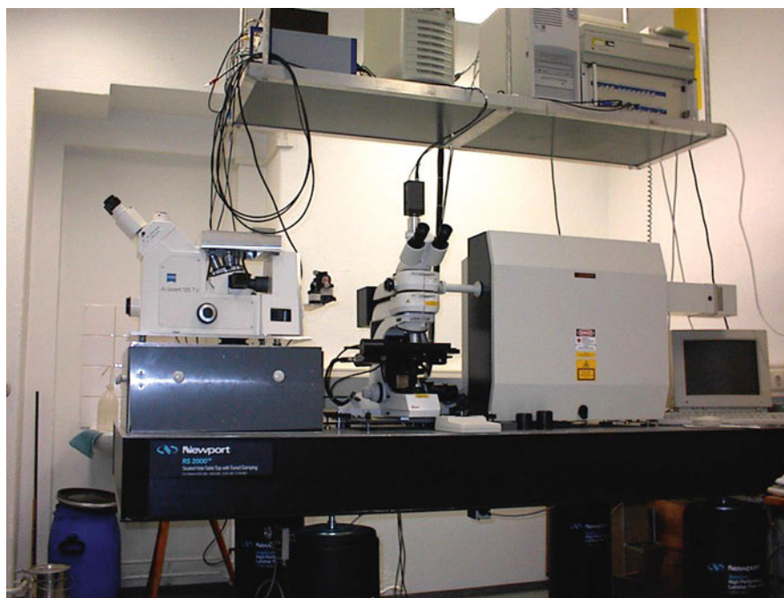
Fig. 8.4 Confocal scanning microscope used for Raman microscopy
